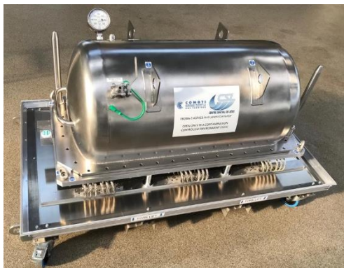
Inner envelope placed on the outer base
